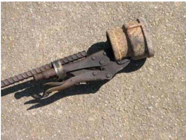
Getting back to the roaring fire, we throw in the pipefittings and wait until they glow. Grabbing one with BBQ tongs, we leave the others to keep heating. After clamping the fitting with the vice grips on the gizmo, we melt some holes until the fitting cools (about 50 holes on a warm day). Then the warm fitting is
